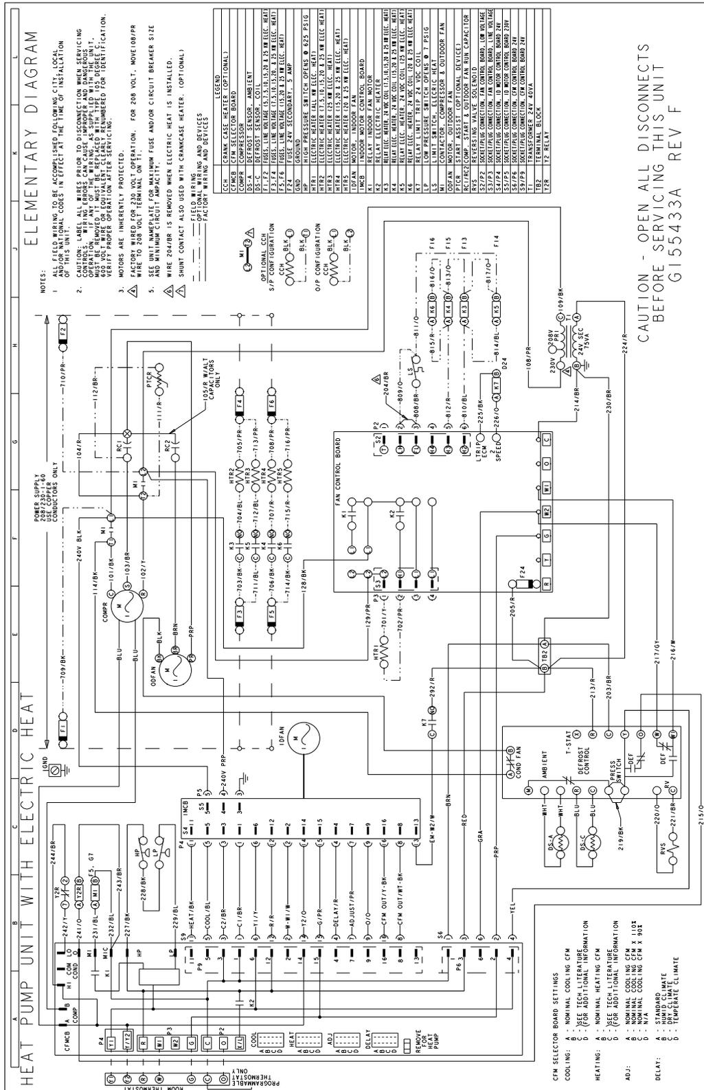
Typical BHX036 Heat Pump 230-3-60 volt Wiring Diagram
