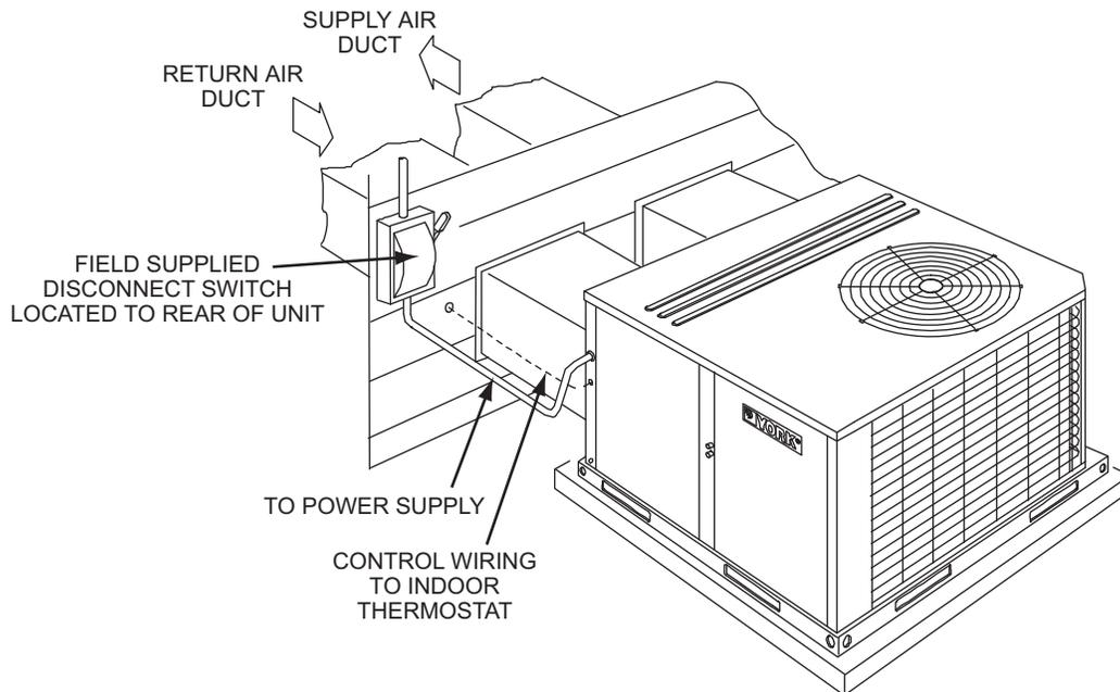
**Unit Typical Roof Curb Installation**
