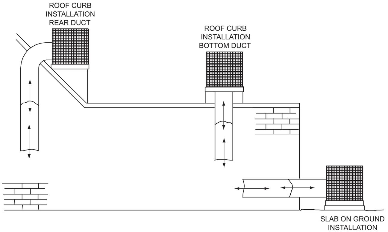
**Unit Typical Slab on Ground Installation**
